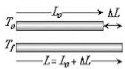
The change in length  $\Delta l$  of almost all solids is directly proportional to the change in temperature  $\Delta T$  as long as is not too large. This means by changing temperature the length also changes, more the change in temperature more is the change in length and vice versa. Sducation (Dustem
